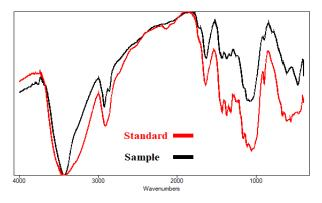
(Fig. 4) The FTIR analysis of tracing paper sample treated with Nanocalcium Hydroxide compared to the control sample
