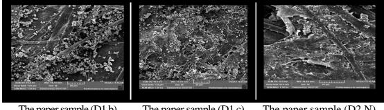
The paper sample (D1.b) treated with Calcium Hydroxide (0.5%) (after aging)
