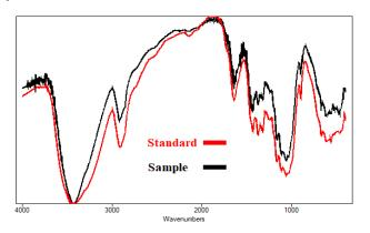
(Fig. 2) The FTIR analysis for the tracing paper sample treated with traditional Calcium Hydroxide (1%) compared to the control sample
