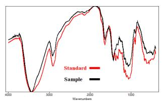
(Fig. 3) The FTIR analysis for tracing paper samples treated with traditional Calcium Hydroxide (1.5%) compared to the control sample.
