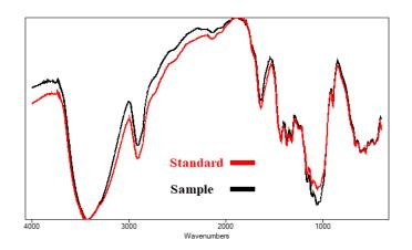
(Fig. 1) The FTIR analysis for tracing paper sample treated with traditional Calcium Hydroxide (0.5%) compared to the control sample
