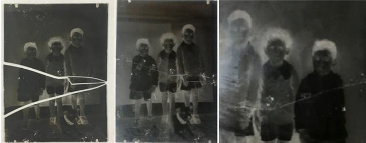
Figure 20. Before assembly (left), after initial assembly (center) and after assembly with four minute epoxy (right)
